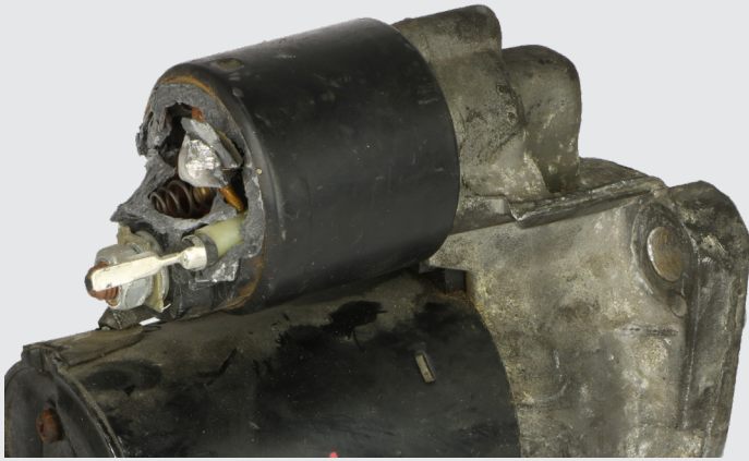
Damaged solenoid / plug
