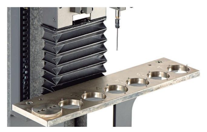
The technological design of the EDR 700 calibration robot enables precise automatic adjustment of any BOSCH, VDO, DENSO and CAT Common Rail injector.
