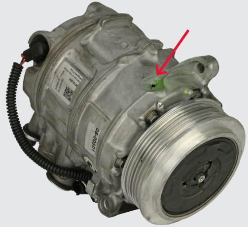
Damaged bracket / fixation
